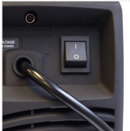
(4) Connect the machine to the correct power supply and switch on the machine using the on/off switch located at the rear of the machine.
