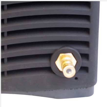
(3) Connect the air supply to the regulator located at the rear of the machine. Set Air Pressure to 0.5MPA (75psi)
