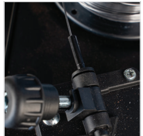
(6) Feed wire over the drive roller into the outlet guide tube, Push the wire through approx 150mm.
