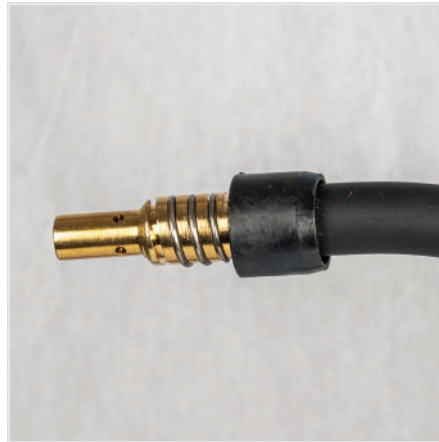
(7) Remove the gas nozzle and contact tip from the front end of the MIG torch.
