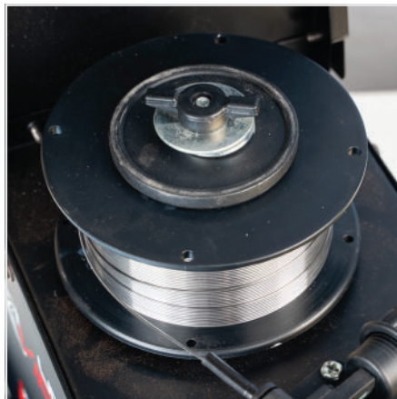
(5) Place wire onto spool holder - (spool retaining nut is left hand thread ) Feed the wire through the inlet guide tube into the drive roller. NOTE: VIPER MIG 120 is not suitable to weld Aluminium as it is a Synergic Welding Machine programmed for Solid Mild Steel wire and Flux Cored (Gasless) wires only.
