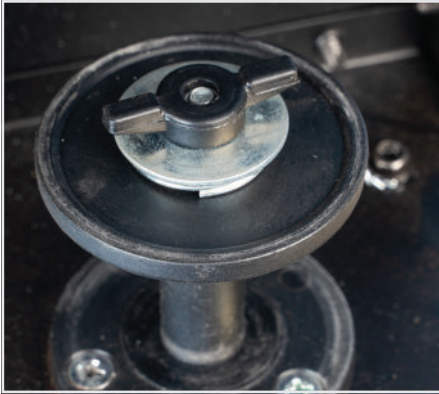
(1) Remove the spool retaining nut.
