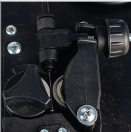
(6) Close down the top roller bracket and clip the pressure arm into place. Apply a medium amount of pressure to the drive roller.
