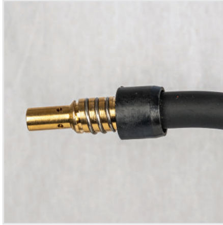
(8) Remove the gas nozzle and contact tip from the front end of the MIG torch.
