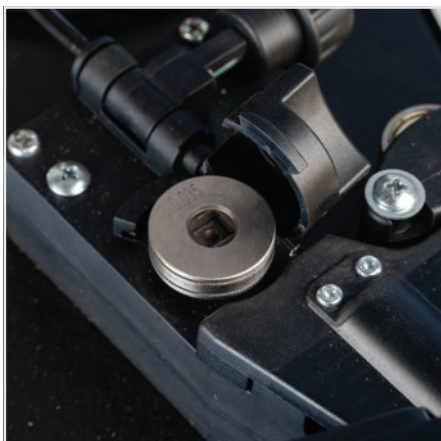
(3) Fit the correct size Knurled drive roller for Gas Less Flux Core wire
