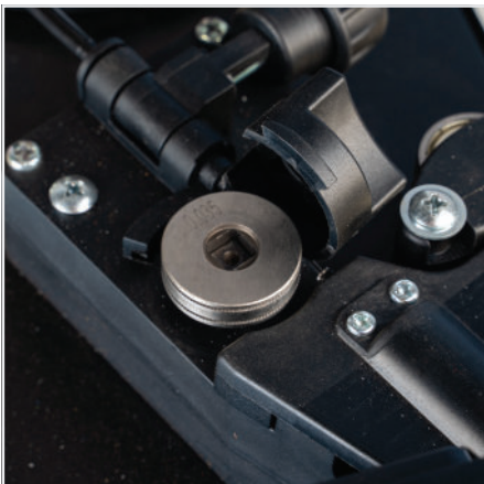
(4) Fit the correct type and size of drive rollers. V Groove for Hard Wires. Knurled for Flux Cored.
