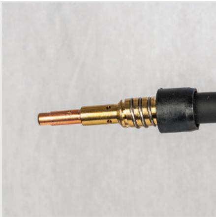
(9) Fit the correct size contact tip over the wire and fasten tightly into the tip holder.
