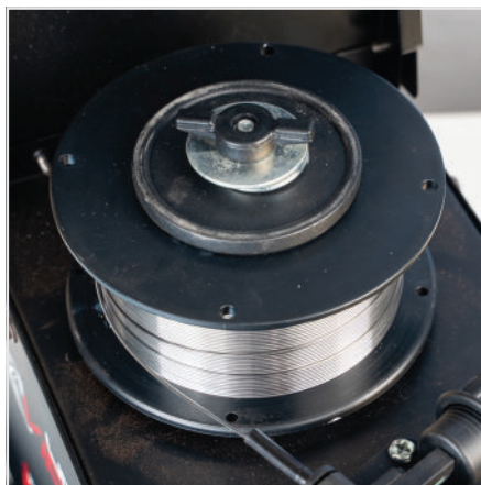
(4) Place wire onto spool holder - (spool retaining nut is left hand thread ) Feed the wire through the inlet guide tube into the drive roller.
