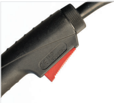
(7) Press and hold the Torch Trigger to feed the wire down the torch cable through to the torch head.
